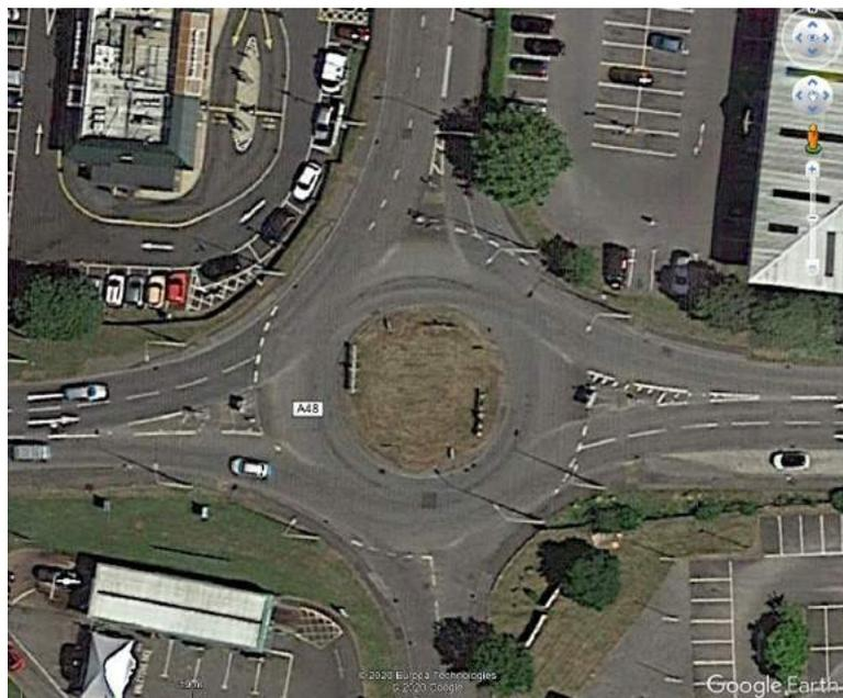
*Image 26 – Pedestrian refuge islands with tactile paving and dropped kerbs on north, east and west arms of Picton Court Roundabout. Missing tactile paving on southern arm (© Google Satellite 6/25/2018)*
