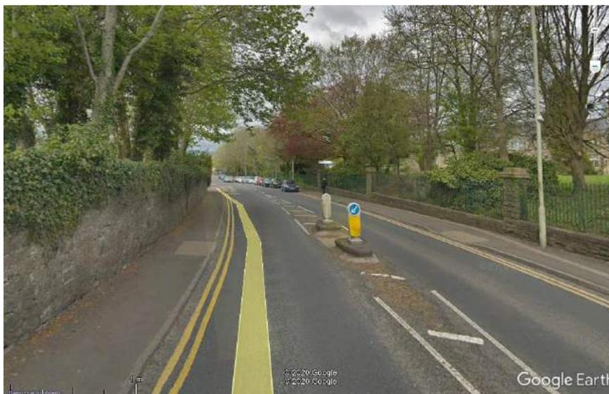
*Image 13 – Pedestrian crossing with tactile paving, dropped kerbs and refuge island. (© Google Streetview 05/18)*
