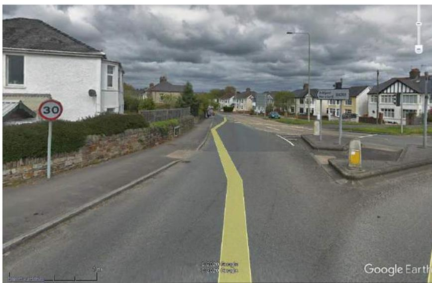
*Image 9 – 30mph speed limit on Ewenny Road north of roundabout towards the town centre. Dropper kerbs, tactile paving and refuge island crossing. (© Google Streetview 05/18)*
