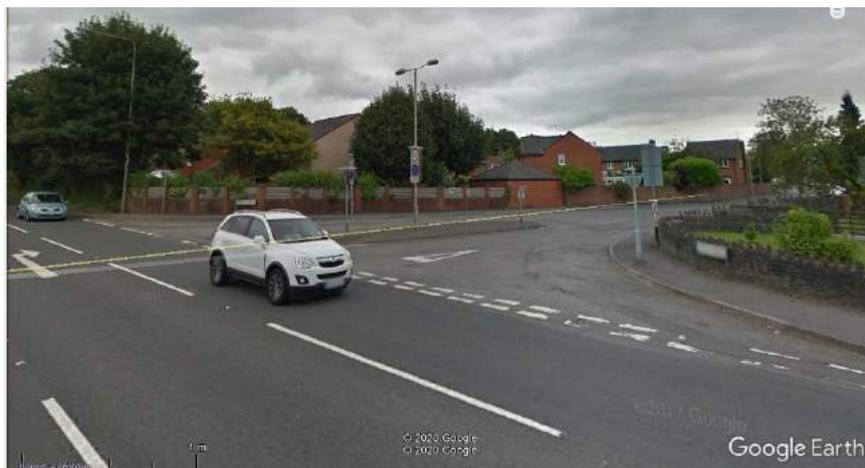
Image 5 – No dropped kerbs and tactile paving crossing. (© Google Streetview 08/16)
