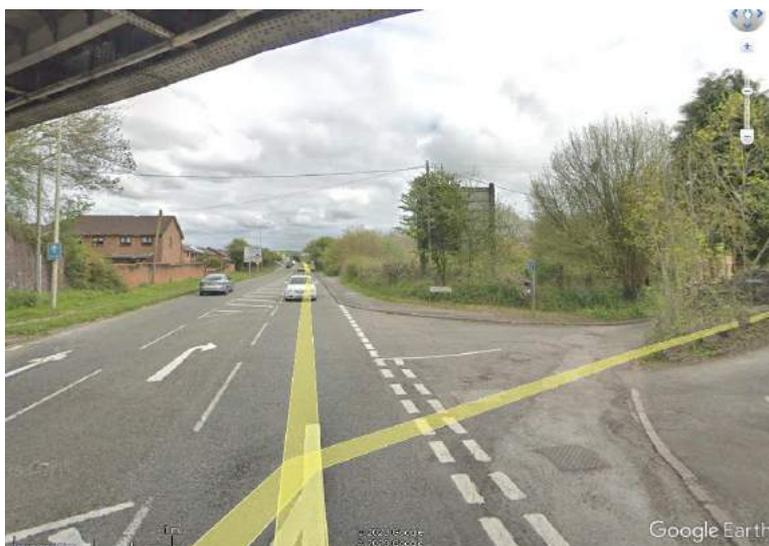
Image 24 – Missing dropped kerbs and tactile paving at Hernston Lane junction (© Google Streetview 05/18)
