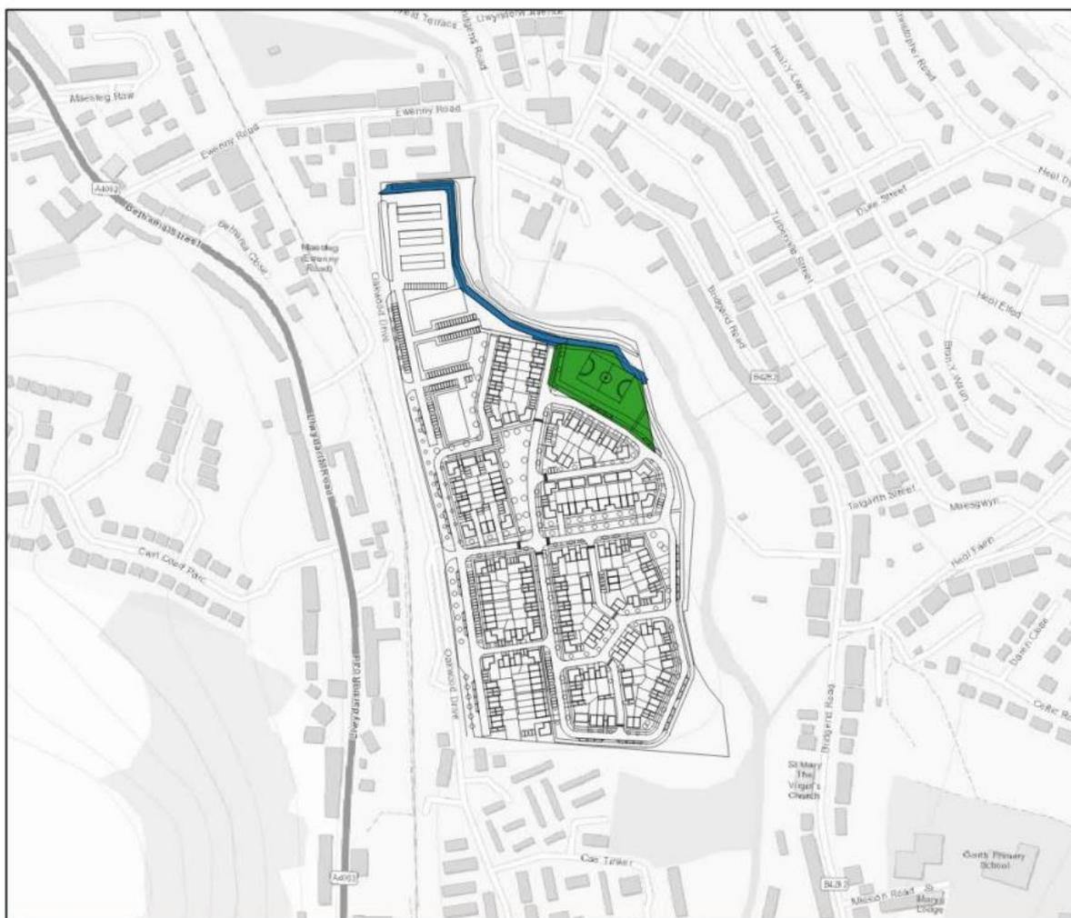
Figure 4-4: Proposed Flood Conveyance Channel and Attenuation (WSP FCA, P. 7)
