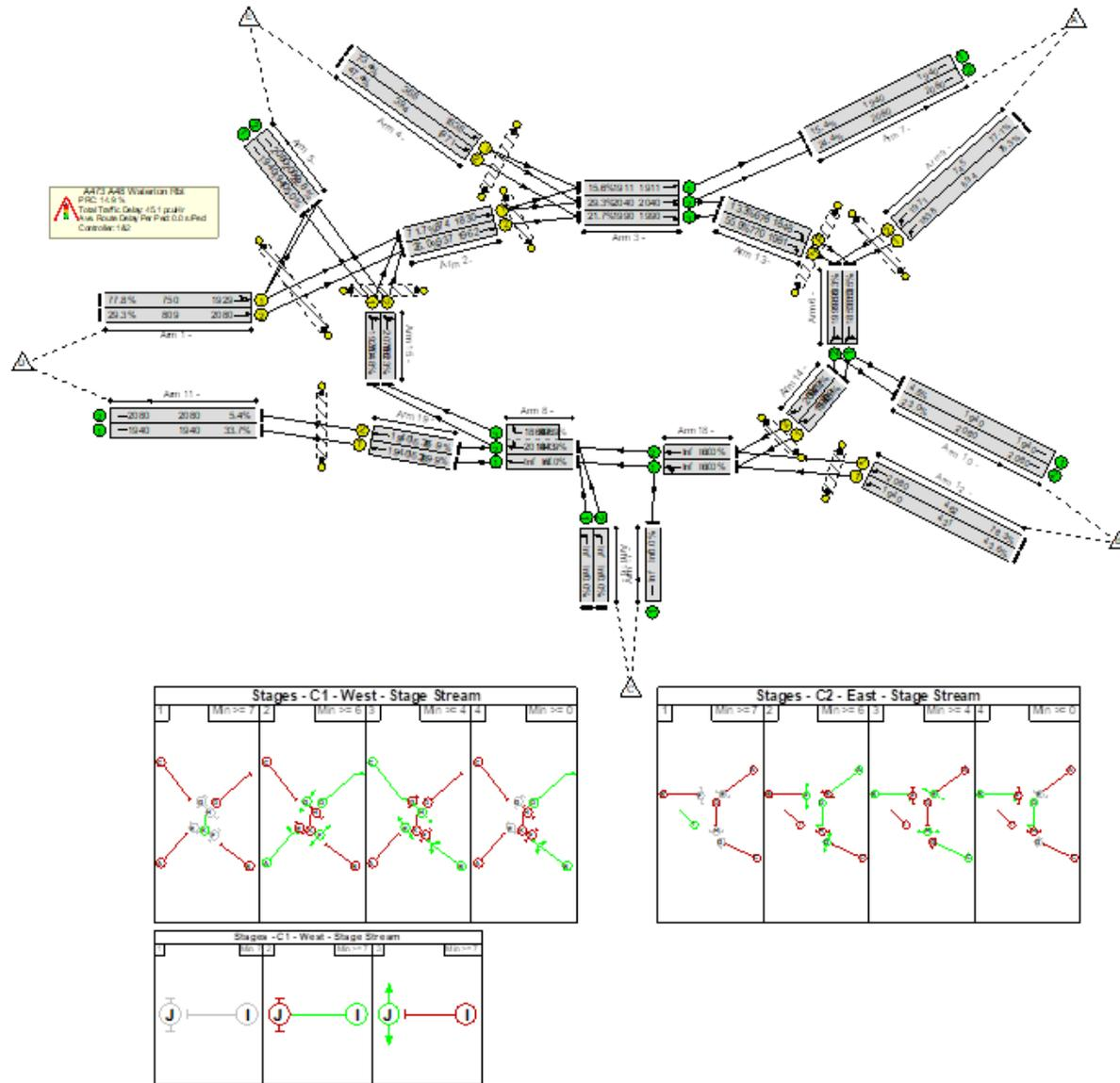
Figure D: Network Layout Diagram, Junction 8
